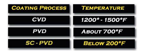
Because of this **ULTRA-LOW** coating temperature, there is no change of material hardness or toughnes and sharp edges can be coated easily.
